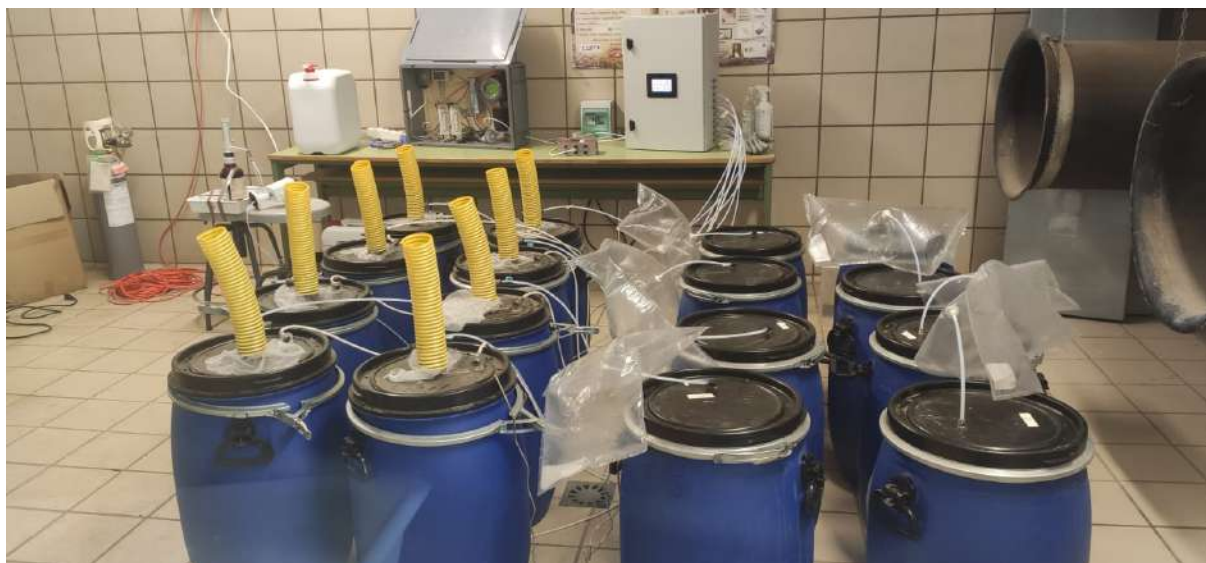
Figure 1. Measuring ammonia emissions from manure treated with different acid levels.
