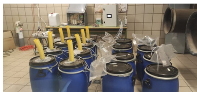
Figure 1. Measuring ammonia and methane emissions from manure treated with different acid levels.
