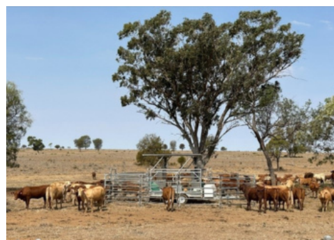
Figure 1. The GreenFeed system (C-Lock Inc.) is used to measure individual methane emission on pasture in Australia. The methane emission is collected while the animal is eating concentrate. (Credit: Sam Clark)
