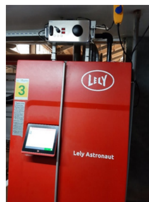
Figure 2. The sniffer methane sensor (Carltech B.V.) connected to the automated milking system on commercial farms in The Netherlands. In The Netherlands 100 commercial farms are equipped with sniffers for routine methane recording (Credit: Anouk van Breukelen)
