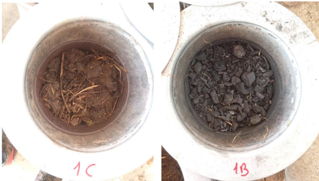
Figure 5 - Image of the collar ring over, respectively, the pot with pure manure (left) and with manure cover with a layer of biochar (right).
